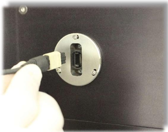
*or CS Raman Spectrometer*, optimal  $f/2.2$  integration is achieved, high signal-to-noise ratios, short acquisition times and repeatable optical coupling is ensured. The keyed multi-fiber connector can only plug-in one-way and “snaps-in” to ensure consistent fiber positioning between the probe and spectrometer. Finally, the Raman Lensed Probe can be outfitted with a removable wand having a 0.25” OD allowing for
